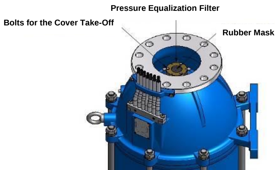
Figure 17 – Pressure Equalization Filter
