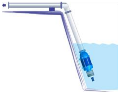
Figure 9 – Amphibious pump working submerged
