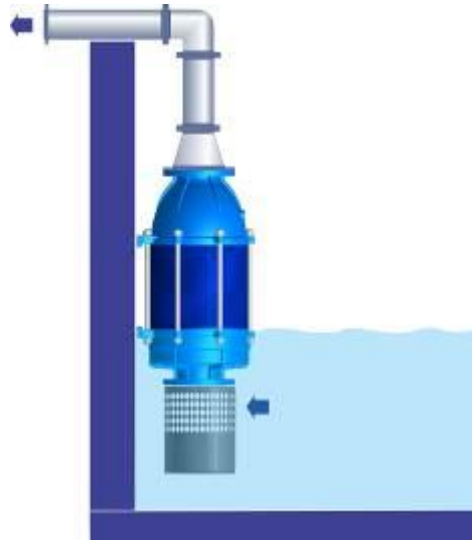
Figure 14 – Pump operating with suction submersed only
